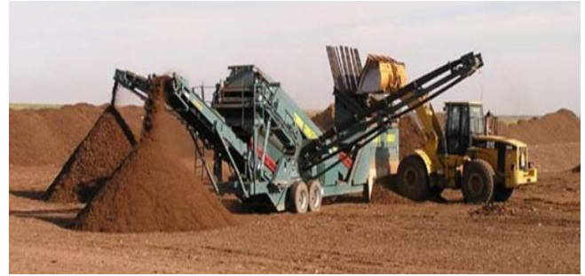
Fig. 4.2. Cure site. Reintroducing oxygen to the pile (left); screening of the finished compost (right)
